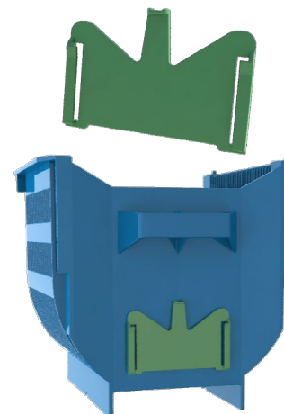
CARD HOLDER-R.1 Welded to Process Boat
