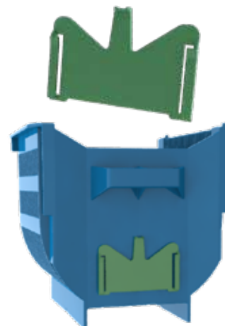
CARD HOLDER-R.1 Welded to Process Boat
